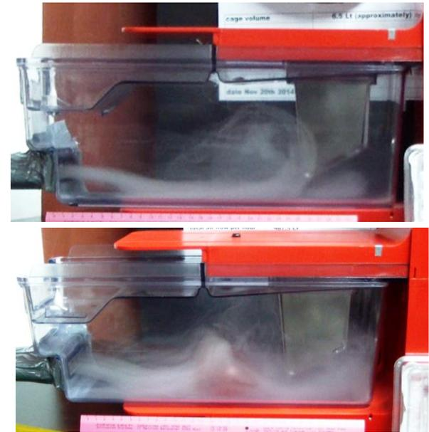
The above pictures are actual airflow in the Airlaw cage. These pictures were taken about 10 seconds after smoke was introduced. Note effect of the dome on the airflow. Cage pressure 1.7 Pascals.
